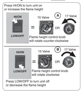
Fig. 2-3 Switch operations
