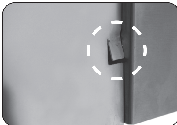
Fig. 24-3 Tab slightly bent in for clearance
