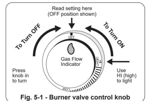
Fig. 5-1 - Burner valve control knob
