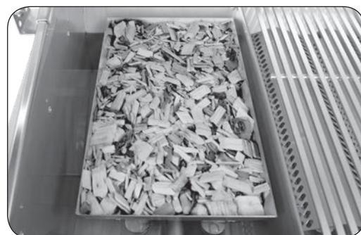
Fig. 35-3 Load wood chips/chunks
