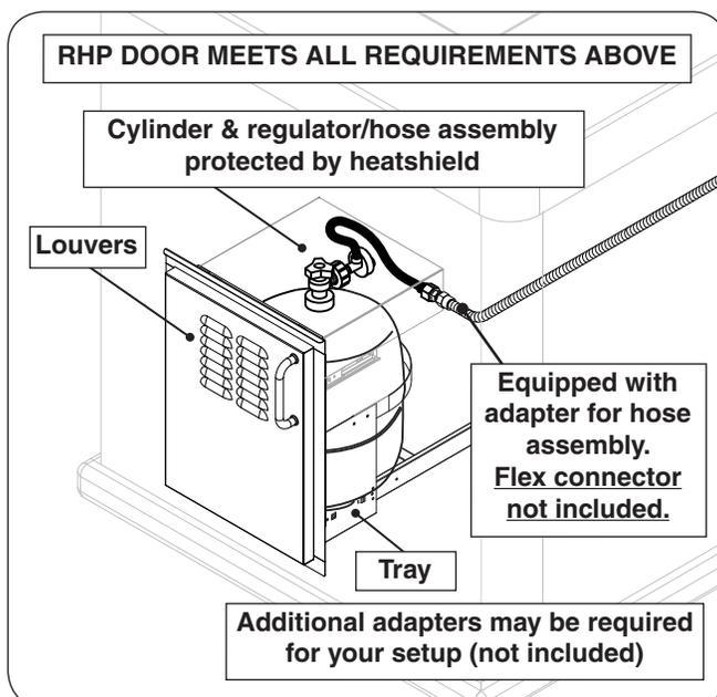
**Fig. 9-3** Optional door w/ tank tray & louvers
