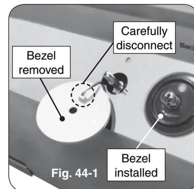
**Important:** When opening, take caution to not damage any wiring.
