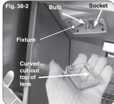
6. Inspect the old bulb for broken glass or filament.
