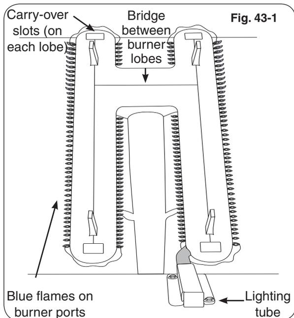
**CAUTION:** Turn all burner control knobs to the **OFF** position and turn off the gas supply at the source before removing or adjusting a burner.
