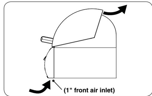
Fig. 12-1 Airflow diagram
