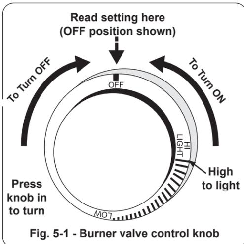
Fig. 5-1 - Burner valve control knob
