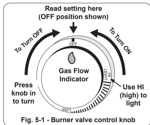
Fig. 5-1 - Burner valve control knob
