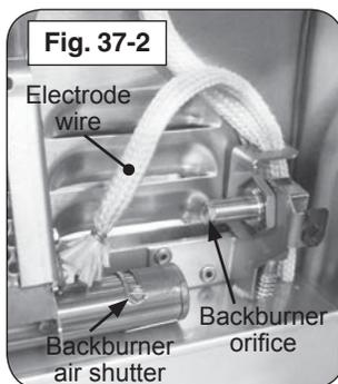
7. Use a  $\frac{3}{8}$ " hex nut driver to remove the exposed orifice. Check orifice. If needed, replace it with the correct orifice for the new gas.
