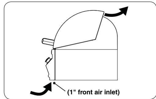
Fig. 12-1 Airflow diagram
