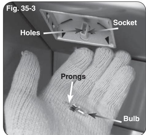
7. Insert the new **12V / 10 watt** halogen bulb into the socket so that both pins slide all the way into the two holes in the bottom of the socket.
