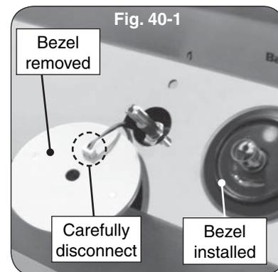
**Important:** When opening, take caution to not damage any wiring.
