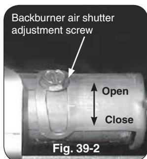
Too large an air shutter opening will allow too much air into the burner, which will cause the flames first to shorten and then to appear to lift up off the ports. For the bottom of the flames to move closer to the ports, close the air shutter more.
