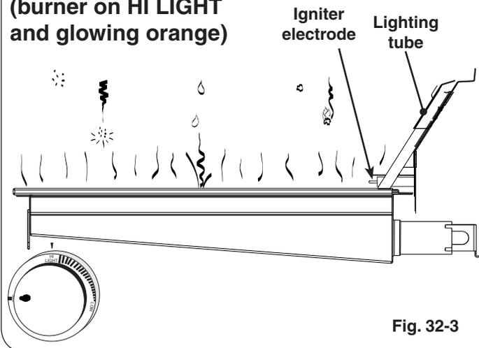
Drips and particles evaporate before hitting infrared burner when cooking at the maximum setting.
