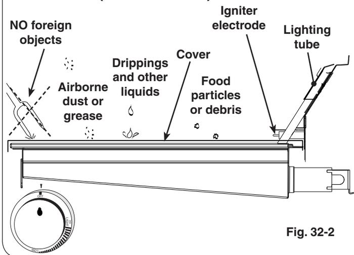
Burner ceramic must be protected with cover when burner is not in use.
