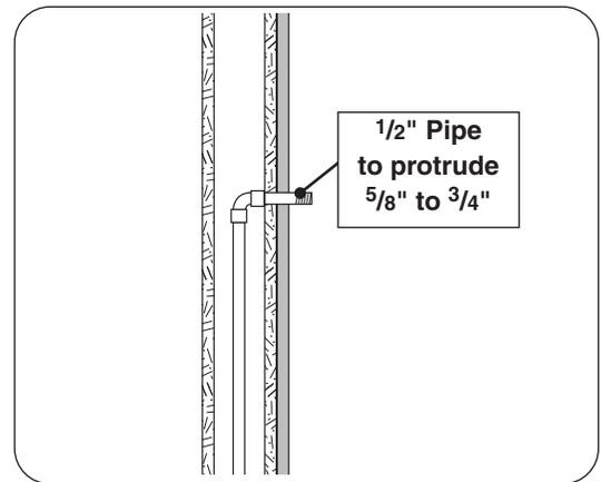
Fig. 1-2 Piping detail
