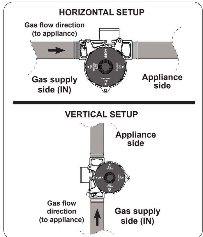
**Fig. 1-2** Automatic timer shut-off valve installation detail
