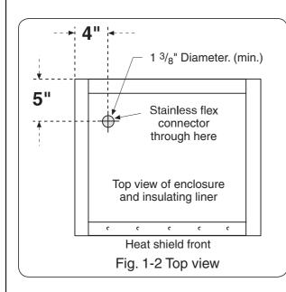
A rigid  $^{1}/_{2}$ " or  $^{3}/_{4}$ " black steel pipe should be used to conduct the gas supply into the enclosure for connection to the outdoor gas appliance. On units with a sheet metal bottom, a 1  $^{3}/_{8}$ " diameter hole set in 4" from the left side and 5" from the rear is provided for plumbing the gas connection (see Fig. 1-2). Use a CSA approved stainless steel flex connector to link the appliance to the gas line.
