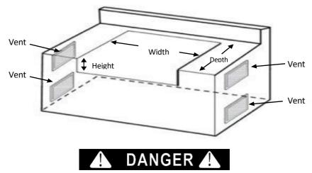
Minimum of 2 vents, but optimally 4 vents, per cabinet that has any sort of gas supply or connection. Each vent must be at least 20 sq in in size and have access to outside/fresh air. Two vents on each side will facilitate and improve airflow and ventilation.
