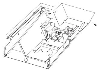
Attach one end of the 34 inch stainless steel flex line to the end of the Side Burner valve. Attach the remaining end of the hose to the "tee" and use two wrenches to tighten the stainless steel flex line connections. One wrench should be used to turn the stainless steel flex line connector while the "tee" or valve is held with the second wrench.
