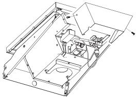
Attach one end of the 34 inch stainless steel flex line to the end of the Side Burner valve.
