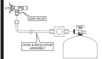
Attach one end of the ten inch stainless steel flex line to the end of the grill's gas valve. Attach the other end of the stainless steel flex line to the brass "tee".
