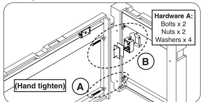
Fig. 7-3 Assemble right side wall and outlet box
