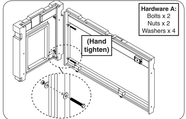
Fig. 7-2 Assemble left side and rear wall
