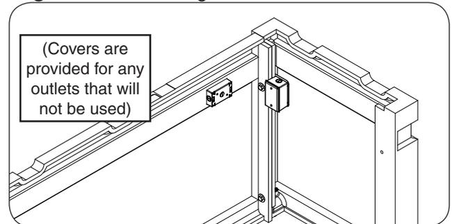
Fig. 7-4 Right side wall and outlet box installed
