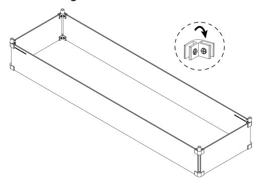
Gently secure all screws (on all brackets)  $^{1}/_{4}$ " to  $^{1}/_{2}$ " turn until panels are secure. DO NOT OVERTIGHTEN.
