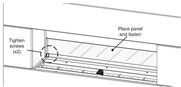
Place one wind guard panel into burner area, ensuring it is centered. While holding, use a  $\frac{5}{16}$ " nut driver and two of supplied screws to fasten panel in place.
