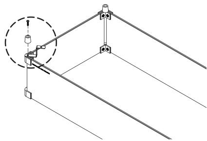
Remove rubber peg from bottom bracket, place mounting bracket, then reinstall rubber peg to bottom bracket.
