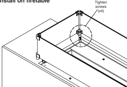
Use a  $^{5}$ /16" nut driver and supplied four screws to fasten guard in place. Start all four screws to ensure guard is properly aligned, then fasten all screws.
