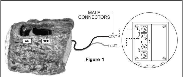
1. Remove the toggle switch connectors from the valve terminal.
